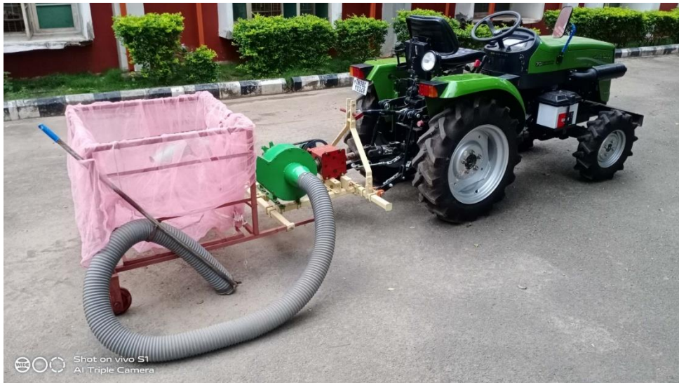
View of the Garbage collector attached to the mini tractor
