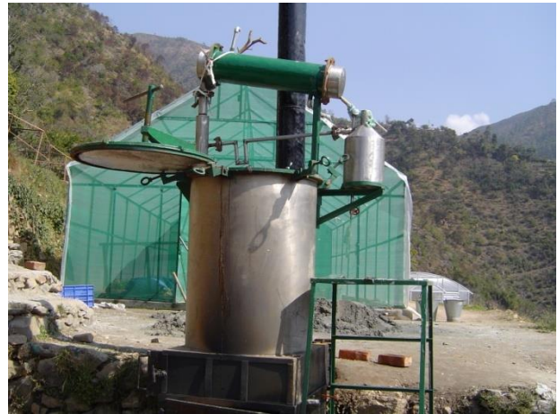
Figure- 6: Distillation unit used for Patchouli oil extraction
